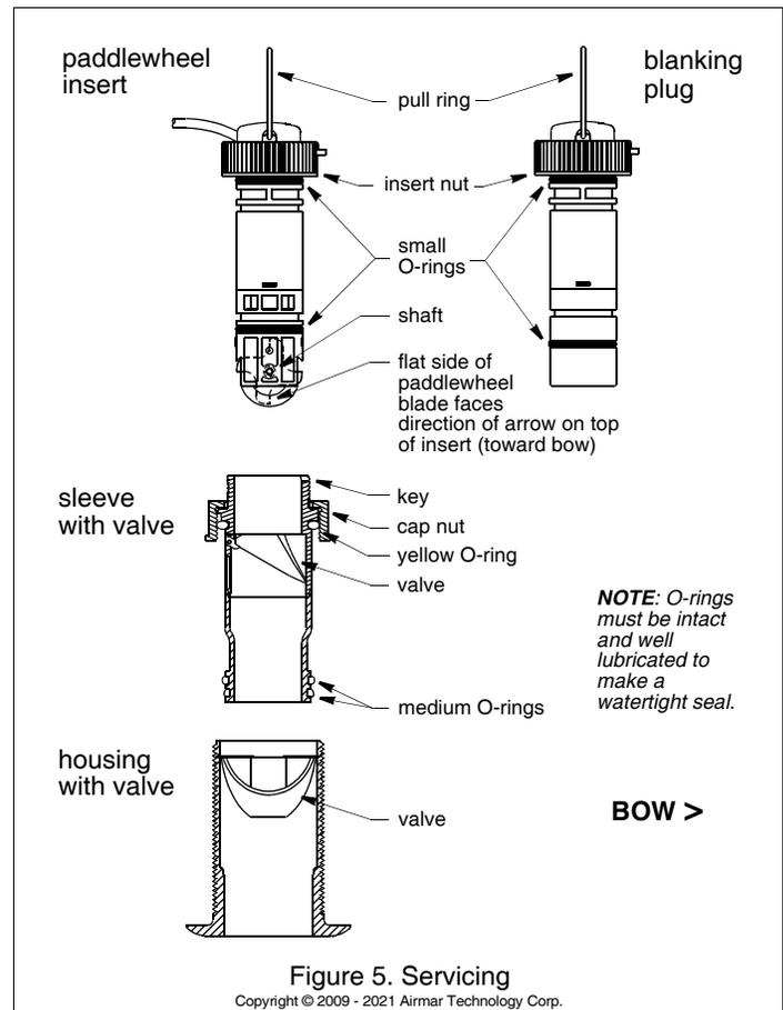
4. All the O-rings must be intact and well lubricated to make a watertight seal. Install two of the small O-rings and lubricate them with the silicone lubricant supplied or petroleum jelly.
