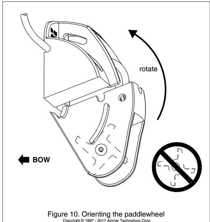
Figure 10. Orienting the paddlewheel
