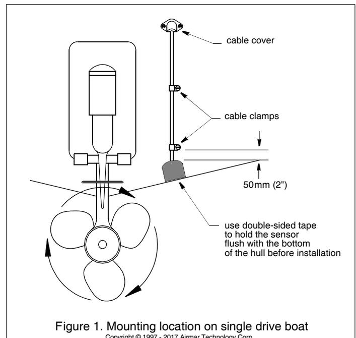
Figure 1. Mounting location on single drive boat
