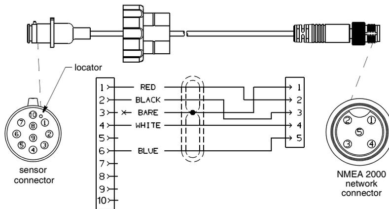
Figure 6. NMEA 2000 Sensor Cable [6m (20') shown]
