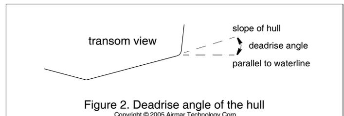
Figure 2. Deadrise angle of the hull
