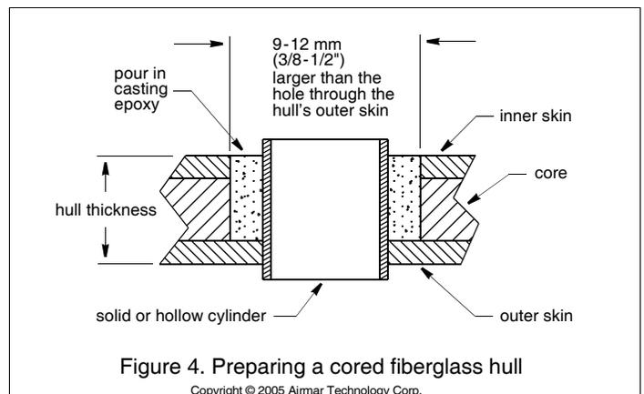
3. From inside the hull, use a 60mm or 2-3/8" hole saw, to cut through the *inner* skin and most of the core. The core material can be very soft. Apply only light pressure to the hole saw after cutting through the inner skin to avoid accidentally cutting the *outer* skin.
