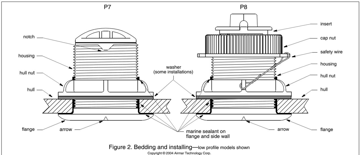
3. Screw the cap nut several turns, then check that the arrow on the insert is still facing forward toward the bow. Continue to tighten the cap nut. **Hand-tighten** only. Do not over tighten.
