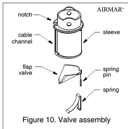
**Warning:** If a new valve assembly is required and not immediately available, the valve sleeve must be reinstalled in the multisensor housing for a watertight seal. Remove the flap valve, spring pin, and spring from the sleeve.
